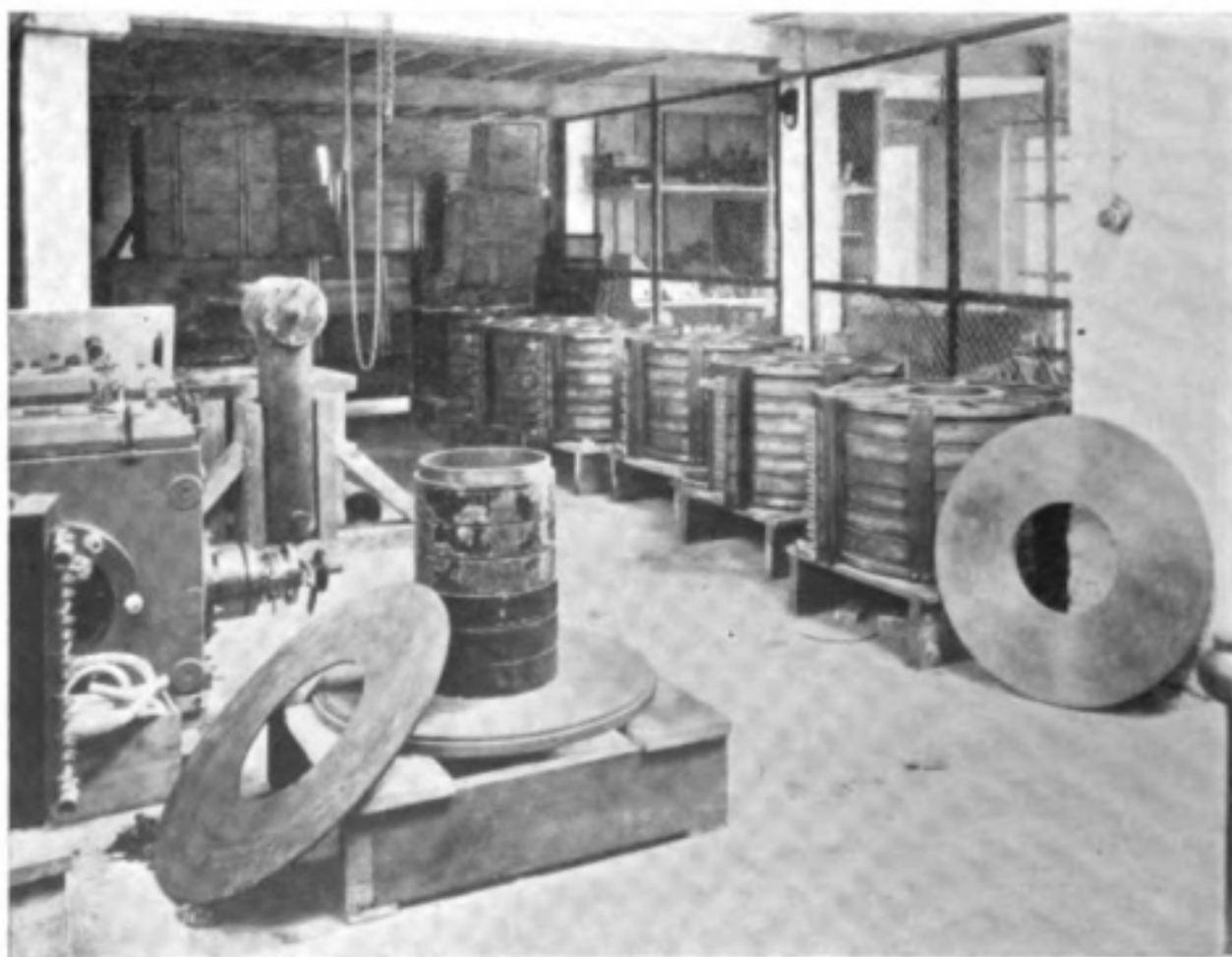
FIG. 12.—Component Parts of one of the 250 kW Arcs during manufacture at works of Messrs. C. F. Elwell, Ltd.
